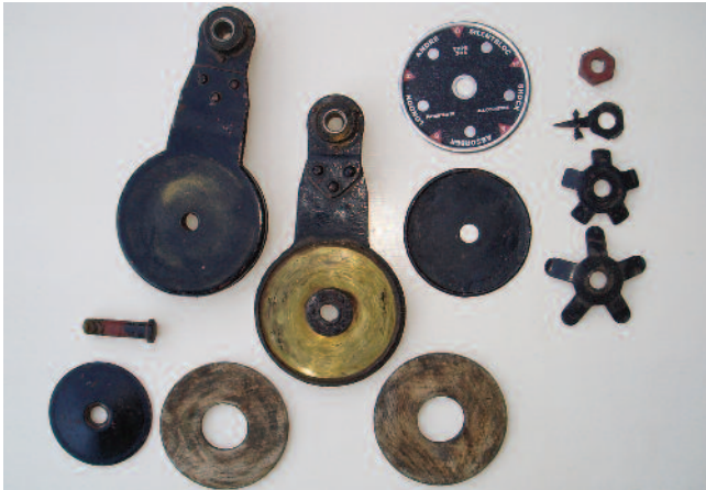
A typical Andre Hartford Shock Absorber as fitted to a P-Type MG (Photo: Digby Gibbs)
